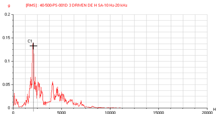
Fig. 11. Value of vibration on different points of the Motor and Pump after maintenance
